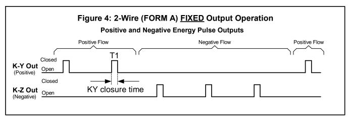
In Signed mode, with a Form A output mode selected, the K-Y output pulse represents positive (or kWh delivered) energy; K-Z output pulse represents negative (or kWh received) energy.
